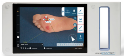
Exact wound measurement and image dimensioning via a state-of-the-art ToF sensor
